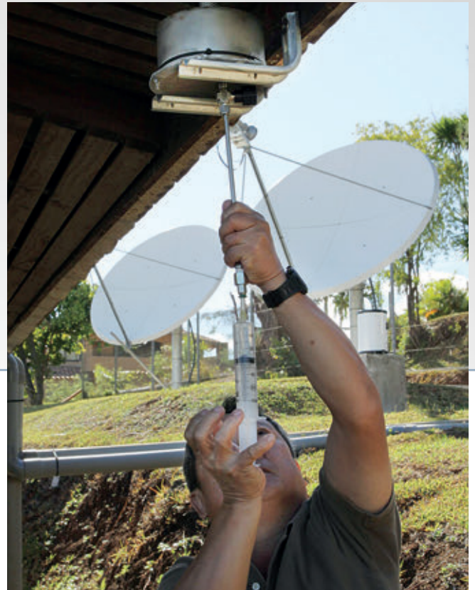
Performing a spike test as part of the certification of the noble gas system at radionuclide station RN27, Papeete, Tahiti, France.
