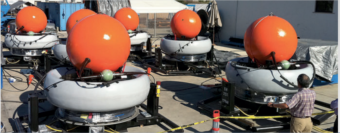
Replacement nodes for the repair and reconstruction of hydroacoustic station HA3 in the Juan Fernández Islands (Chile).
