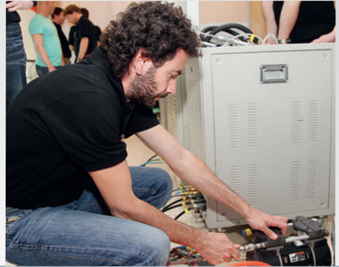
Surrogate inspectors at training courses in China in 2013: troubleshooting (left) and operating the XESPM xenon detection system.
