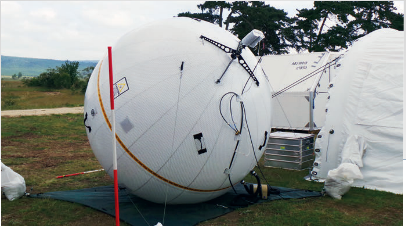
GATR terminal, which was successfully deployed during the build-up exercises and will be used during the Integrated Field Exercise in 2014.
