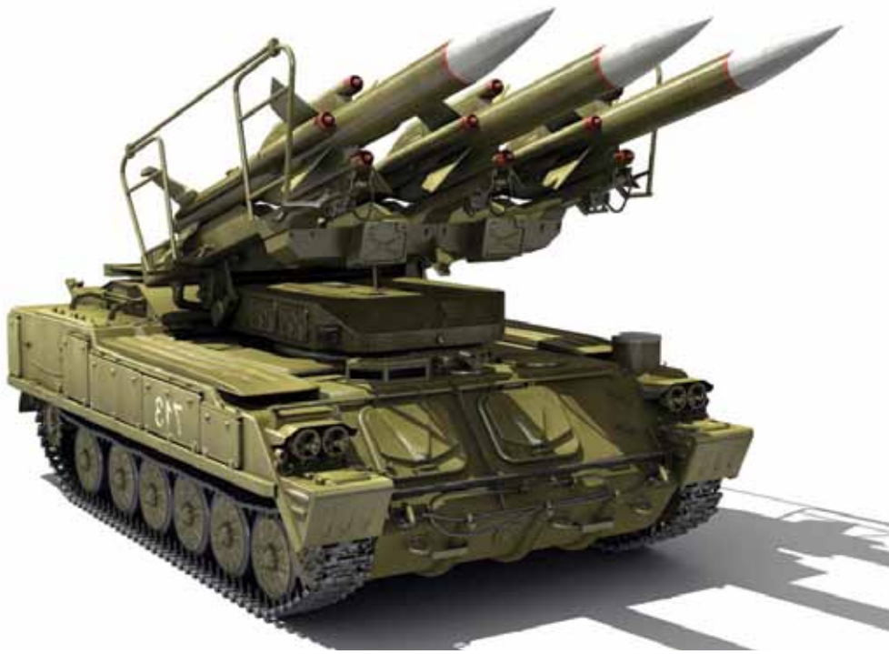
Russian SA-6 GAINFUL is a two stage, solid-fuel, low-altitude surface-to-air missile. Photo courtesy of weapons.technology.youngster.com
