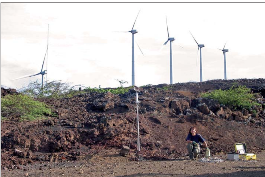
PTS STAFF MEMBER PERFORMING NOISE STUDY IN FRONT OF WIND GENERATORS, MARCH 2005, ASCENSION ISLAND
