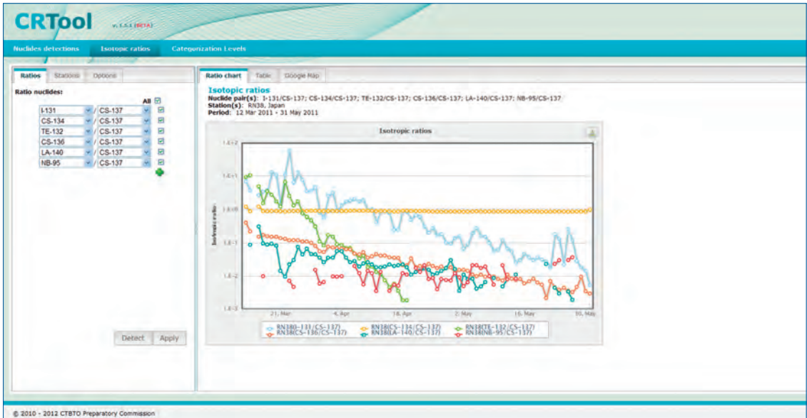
Screenshot of the display produced by CRTool of the evolution of the activity of concentration of several nuclides recorded at radionuclide station RN38, Takasaki, Gunma, Japan, after the Fukushima nuclear power plant accident.
