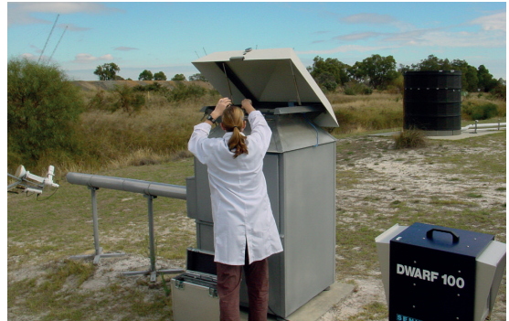
Changing a filter at radionuclide station RN10, Perth, WA, Australia.
