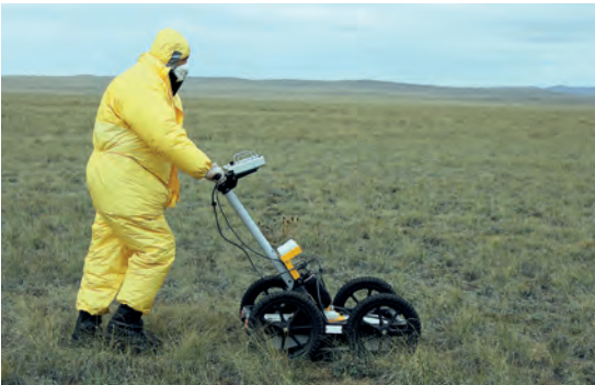
A ground penetrating radar unit is used to detect changes in underground structures during IFE08.
