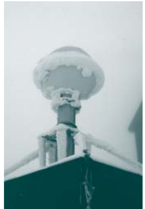
FIGURE 2: ICE RIMING UNDER NATURAL ENVIRONMENTAL CONDITIONS AT SONNBLICK (AUSTRIA)
