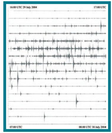
FIGURE 1:SEISMIC PLOT SHOWING THE SEISMIC ACTIVITY RECORDED BETWEEN 16:00 UTC ON 29 JULY 2004 AND 08:00 THE NEXT DAY. THE DATA SHOWN ARE FROM THE VERTICAL COMPONENT OF H09W1. EACH LINE REPRESENTS DATA COLLECTED OVER ONE HOUR; 16 CONSECUTIVE HOURS OF DATA ARE SHOWN; DATA ARE PLOTTED AT THE SAME AMPLIFICATION.
