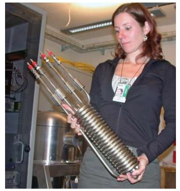
A DETACHED HELICAL XENON GAS ADSORPTION COLUMN WHICH FORMS PART OF THE COMPLETE SAMPLE PURIFICATION SYSTEM
