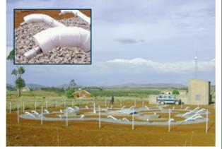
VIEW OF WIND NOISE REDUCING PIPE ARRAY AT AN ARRAY ELEMENT OF INFRASOUND STATION IS33, ANTANANARIVO, MADAGASCAR. INSET: INLET PORTS OF PIPE ARRAY.
