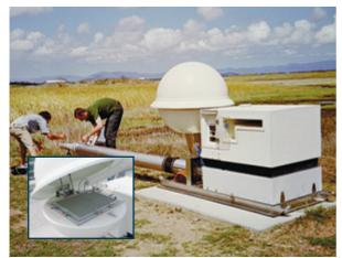
MANUAL AIR SAMPLER AT RN6. INSET: AIR SAMPLER OPEN TO CHANGE FILTER.
