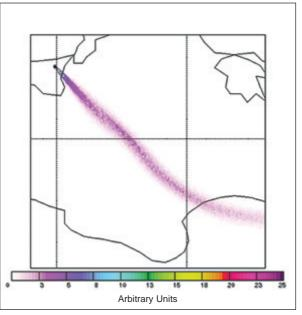
SIMULATION BY THE PTS ATMOSPHERIC TRANSPORT MODELLING TOOL OF THE PLUME CONCENTRATION FOR THE TIME AT WHICH THE SATELLITE IMAGE WAS TAKEN.
