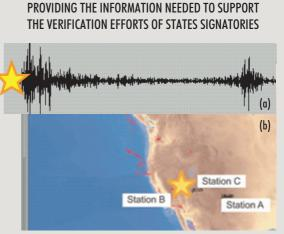
IMS stations detect an event (a), and the IDC analyses waveforms and produces a solution (origin time, location, depth, magnitude) for the event (b).
