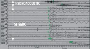
SIGNALS PRODUCED BY AN EARTHQUAKE IN INDONESIA AND RECORDED BY STATIONS FROM DIFFERENT MONITORING TECHNOLOGIES.
