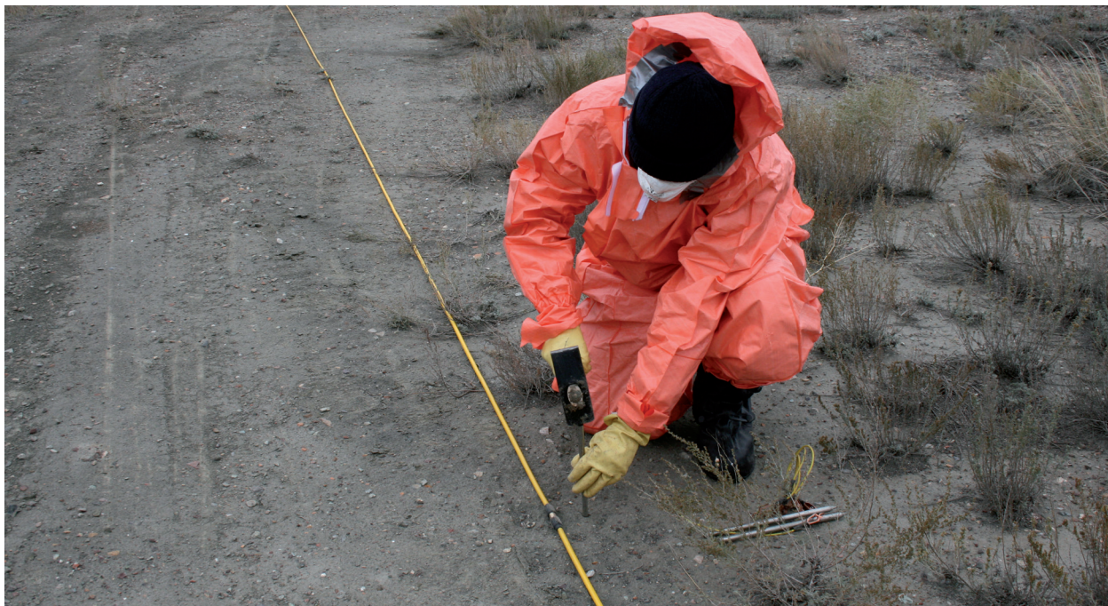
An OSI inspector prepares to measure the electrical conductivity of the ground to identify metal objects or other disturbances.
