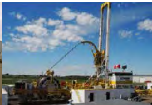
Coiled tubing drill rigs are a "state of the art" drilling system which requires less infrastructure than a rotary drilling rig and can be adapted to many varying site conditions. These rigs are available in various sizes to meet many drilling requirements. Instead of utilizing a drill string that is made up of sections of pipe, a coiled tubing drill rig continuously advances tubing from a large drum which follows a drill bit that is rotated by the circulating drilling fluid.
