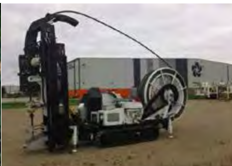
Coiled tubing drill rigs are a "state of the art" drilling system which requires less infrastructure than a rotary drilling rig and can be adapted to many varying site conditions. These rigs are available in various sizes to meet many drilling requirements. Instead of utilizing a drill string that is made up of sections of pipe, a coiled tubing drill rig continuously advances tubing from a large drum which follows a drill bit that is rotated by the circulating drilling fluid.
