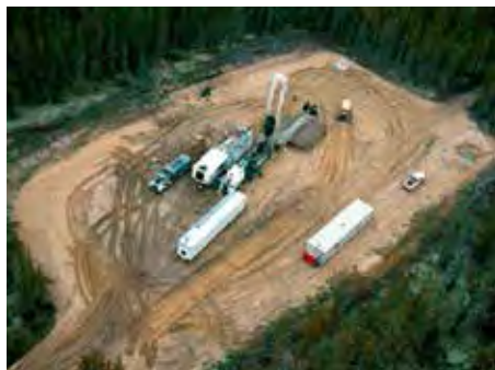
Coiled tubing drill rigs are a "state of the art" drilling system which requires less infrastructure than a rotary drilling rig and can be adapted to many varying site conditions. These rigs are available in various sizes to meet many drilling requirements. Instead of utilizing a drill string that is made up of sections of pipe, a coiled tubing drill rig continuously advances tubing from a large drum which follows a drill bit that is rotated by the circulating drilling fluid.
